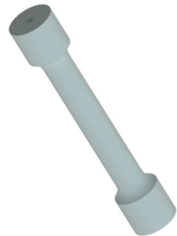
Fig. 3. Blank bar for the tensile test
