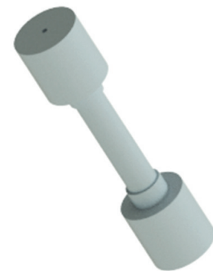
Fig. 4. Blank bar for the creep test
