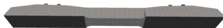
Fig. 2. Under Sleeper Pad - partially covered bottom surface of the sleeper (in the area of the main transmission of vertical pressure) [1].
