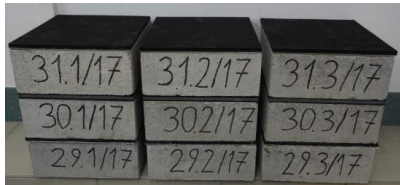
Fig. 5. USP test samples: RUB7(29.1-3), PUR7(30.1-3), RUB9(31.1-3) tested at the Warsaw University of Technology.
