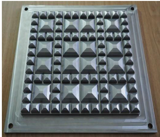
Fig. 7. GBP plate used to tested USP pads in laboratory stand at the Warsaw University of Technology (top view).
