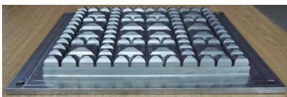
Fig. 6. GBP plate used to tested USP pads in laboratory stand at the Warsaw University of Technology (side view).
