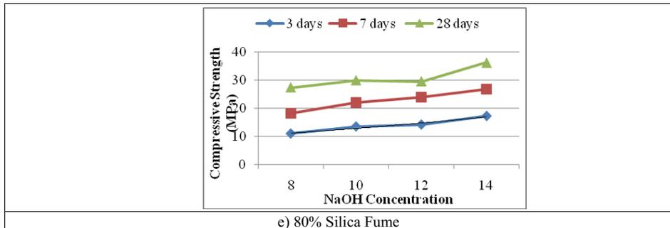
Fig. 3.2 Relationship between Compressive Strength of HCFA Geopolymer Mortar and Silica Fume
