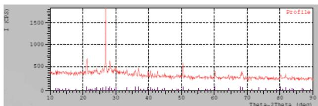
Fig.3.4 X-Ray Diffractogram of Geopolymer Mortar 60% HCFA, 40% silica fume (14FS<sub>40</sub>)
