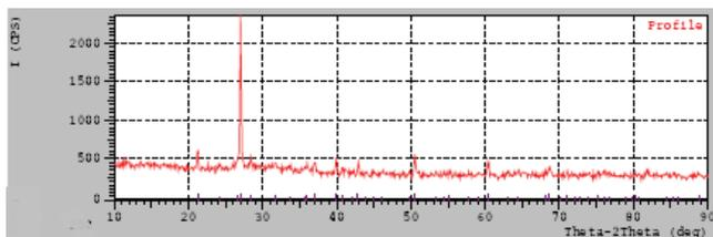
Fig.3.3 X-Ray Diffractogram of Fly ash Geopolymer Mortar 100% HCFA (14FS<sub>0</sub>)
