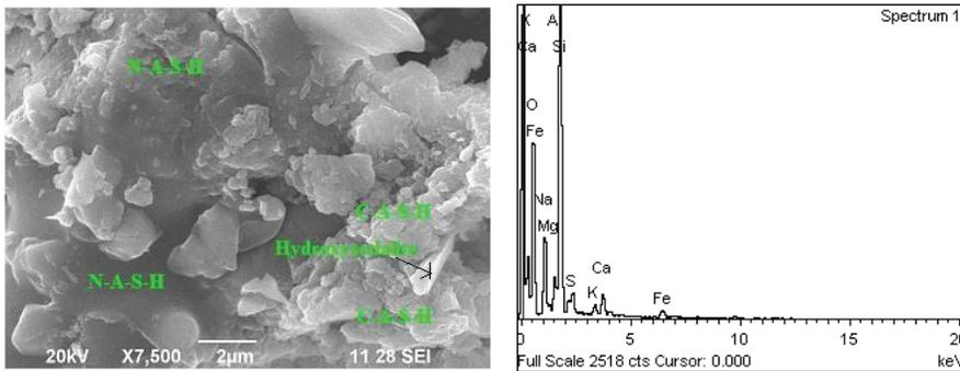
Fig.3.6. SEM-EDAX image of specimen 14FS<sub>40</sub>, mortar cube 14M of NaOH 40% Silica fume 60% HCFA
