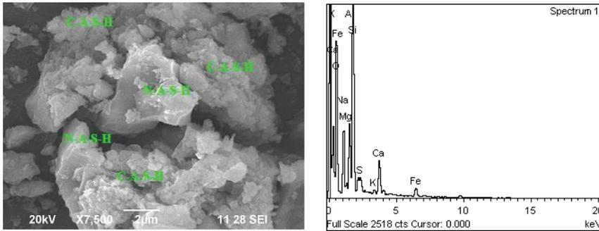
Fig.3.5. SEM-EDAX image of specimen 14FS<sub>0</sub>, mortar cube 14M of NaOH, 100% HCFA
