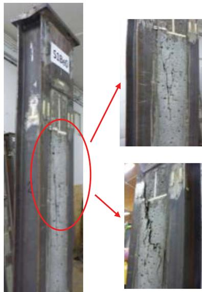
Fig. 3. Example of failure mode (I) for test specimen S1Be0: (a) crushed concrete on the more compressed side; (b) crushed concrete on the less compressed side
