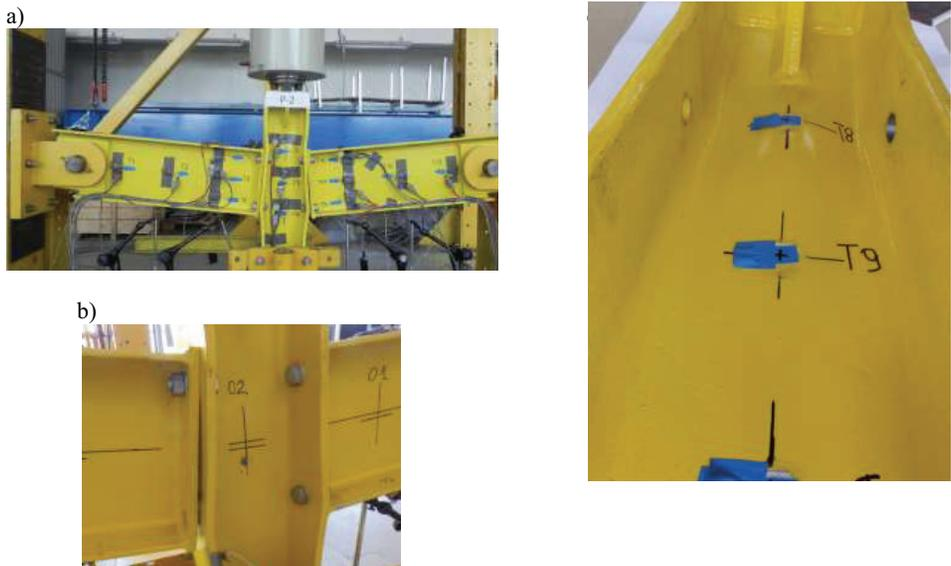
Fig.12. P-2 specimen: a) view before failure, b) failure mode of specimen, c) column view after test
