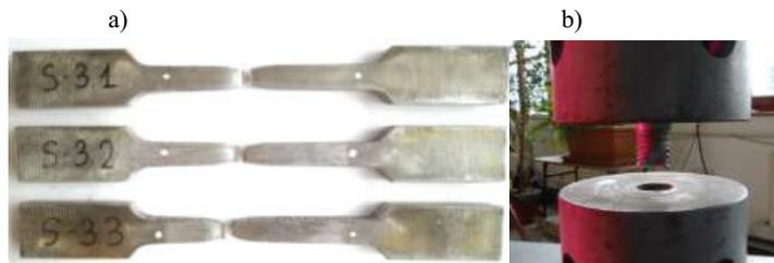
Fig. 7. View: a) material coupon after test, b) bolt after test
