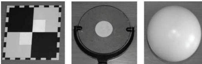
Fig. 3. Targets: (a) b&amp;w, (b) HDS, (c) Faro sphere
