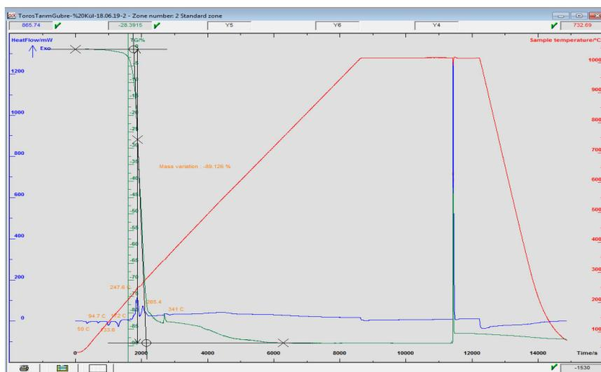
Fig. 12. TGA analysis of 0.01% polyethylene glycol and 0.01% carboxymethyl cellulose added ammonium nitrate
