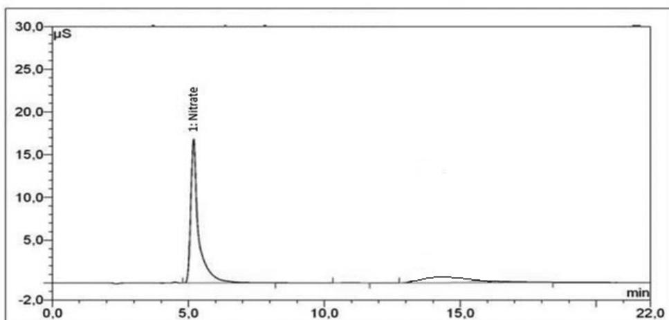
Fig. 3. Ion chromatography of ammonium nitrate with 0.01% polyethylene glycol additive
