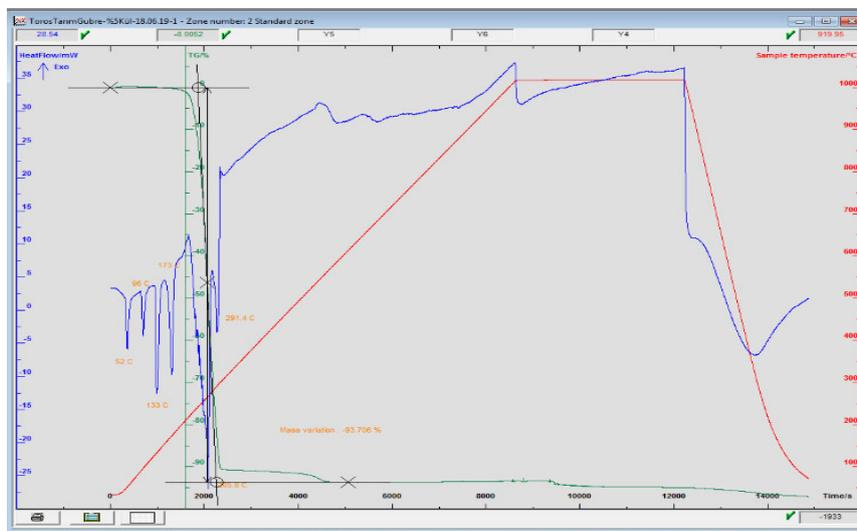
Fig. 10. TGA analysis of ammonium nitrate with 0.01% polyethylene glycol additive
