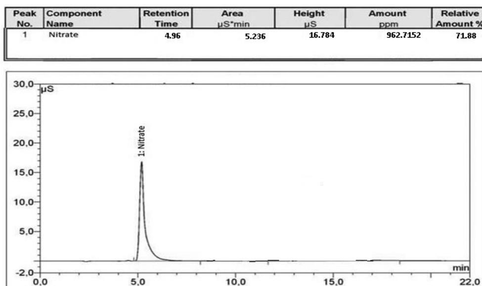
Fig. 5. Ion chromatography of 0.01% polyethylene glycol and 0.01% carboxymethyl cellulose added ammonium nitrate
