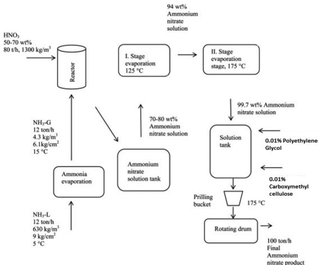
Fig. 1. Ammonium nitrate production with two-stage evaporation method (Gezerman, 2020)
