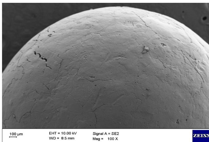
Fig. 7. SEM image of ammonium nitrate with 0.01% polyethylene glycol additive
