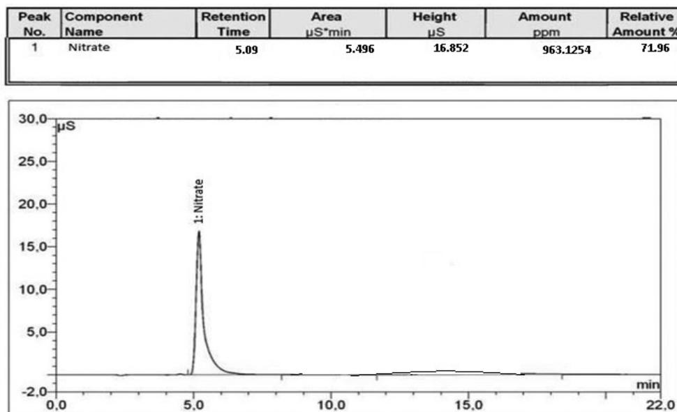
Fig. 4. Ion chromatography of ammonium nitrate with 0.01% carboxymethyl cellulose
