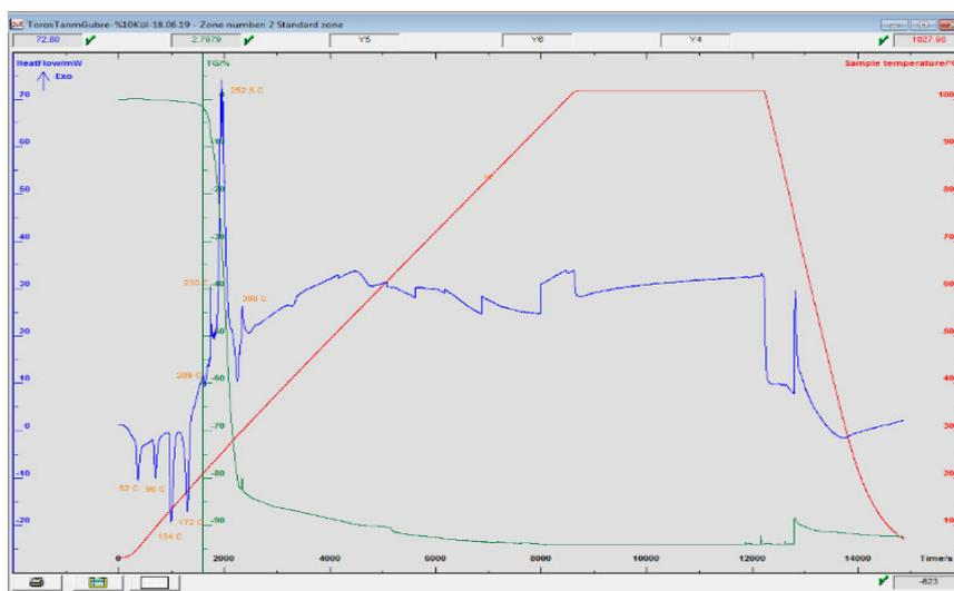
Fig. 11. TGA analysis of 0.01% carboxymethyl cellulose added ammonium nitrate
