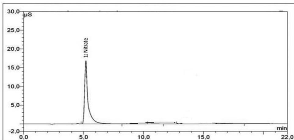
Fig. 2. Anion analysis in ion chromatography of pure ammonium nitrate
