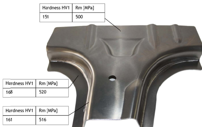
Fig. 6. Strength properties of the lower part of the B-pillar (process without the participation of the lower blankholder in the forming process, as presented in Fig. 3)
