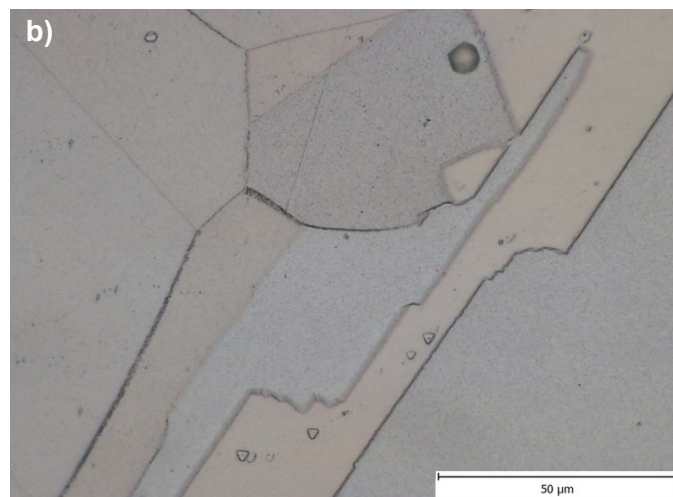
Fig. 10. Grain boundaries with and without fine elements in steel X15CrNiSi 20-12; a) 900°C, b) 1200°C
