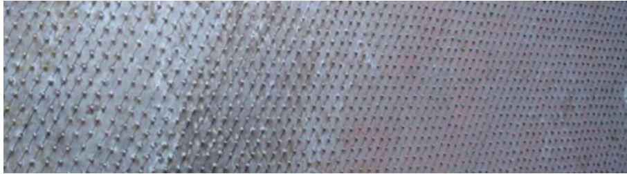
Figure 4: Photograph of spherical ball roughened absorber.
