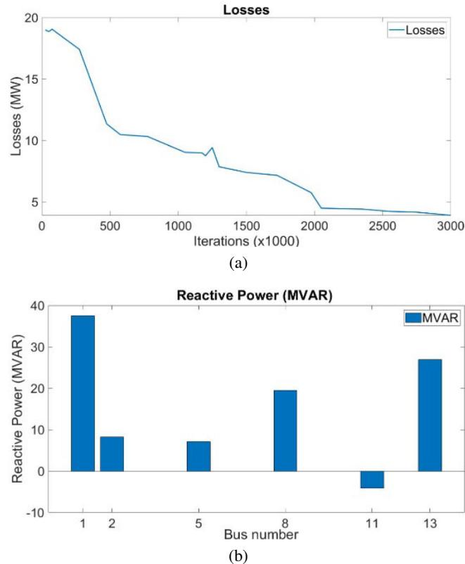
Fig. 3. Losses reduction (30 – bus) (a); reactive power at generating buses (30 – bus) (b)
