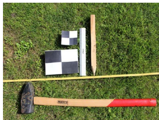
Photo 1. Tools for stabilizing border points (phot. K. Ożóg)
