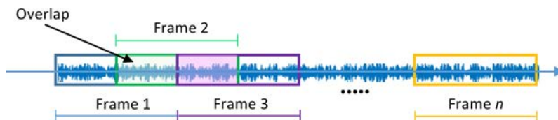
Fig. 4. Windowing is applied to minimize the discontinuities at the edge of each frame.
