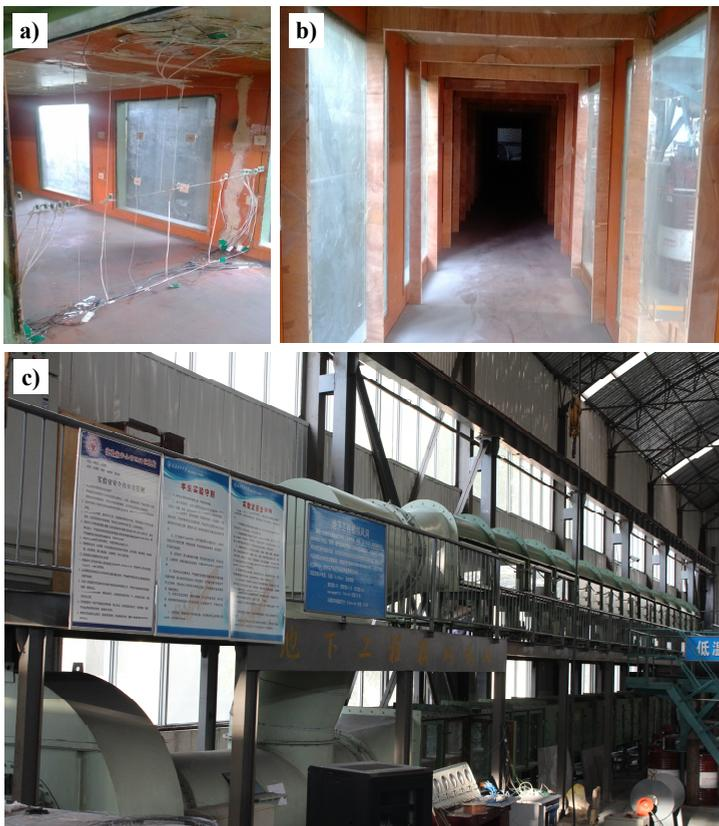
Fig. 7. Pictures of underground engineering simulation tunnel. a) Picture of engineering simulation tunnel, b) I-steel simulation supporting roadway, c) Test measuring points of airflow velocity in boundary layer
