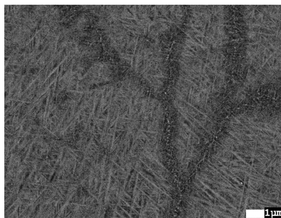
Fig.6. Microstructure of the titanium particle center (SEM)
