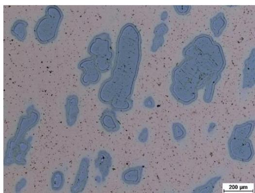
Fig.4. Microstructure of sintered compact obtained for Cu+ 10 % of Ti
