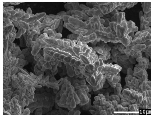
Fig.1. Electrolytic copper powder (SEM)
