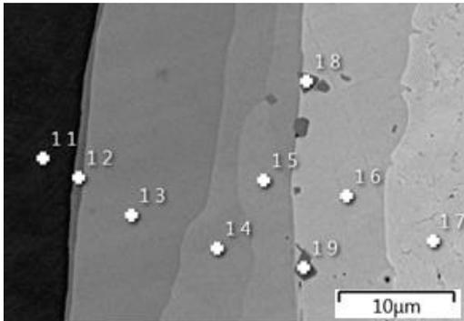
Fig.8. Examples of points where EDS analyses were taken
