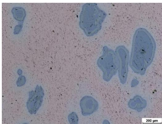
Fig.3. Microstructure of sintered compact obtained for Cu+ 5 % of Ti
