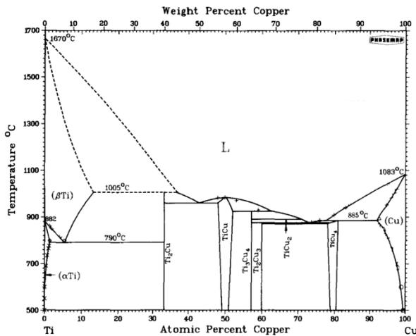
Fig.7. Ti- Cu binary phase diagram [20]
