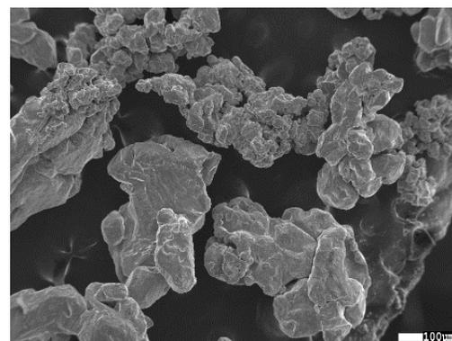
Fig.2. Titanium powder (SEM)
