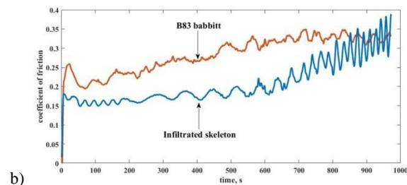
Fig. 7 Pure babbitt vs infiltrated skeleton subjected on a load of 50N: (a) linear wear, (b) coefficient of friction
