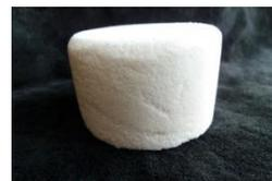
Fig. 2. Optical image of sintered salt preforms with  $\text{Al}_2\text{O}_3$  as reinforcing phase
