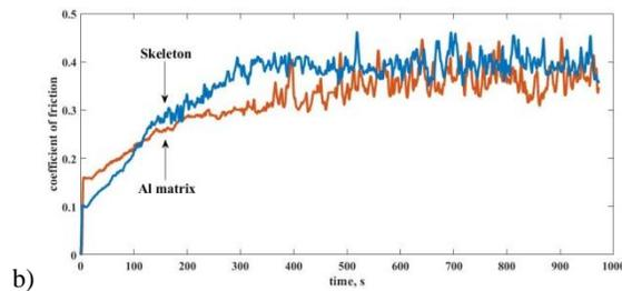
Fig. 8 Al matrix vs skeleton subjected on a load of 50N: (a) linear wear, (b) coefficient of friction.
