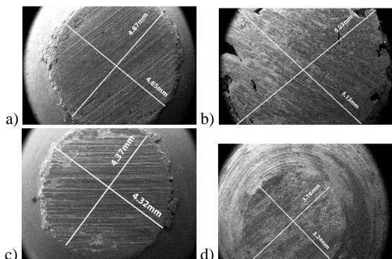
Fig. 6. SEM images of wear scar diameter measurement: (a) Al-alloy matrix, (b) Skeleton, (c) Pure babbitt, (d) Infiltrated skeleton
