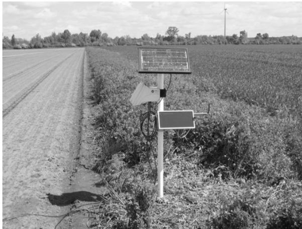
Fig. 2. Soil moisture measurement: logger station from Sentek's EnviroSCAN and GSM modem
