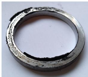
Fig. 5. Steel ring sample after wear test
