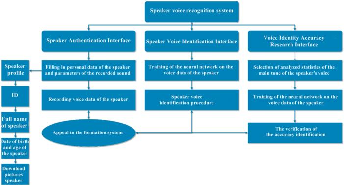
Fig. 3. Structural diagram of voice recognition system speaker
