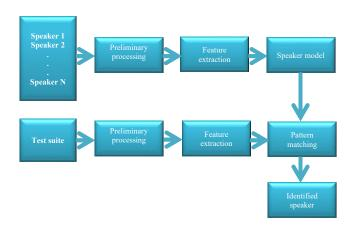
Fig. 1. Basic system of speaker identification
