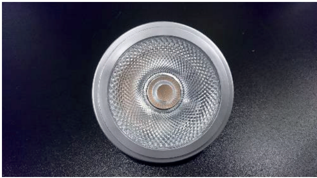
Fig. 3. Spot LED lamp 11.5 W being tested
