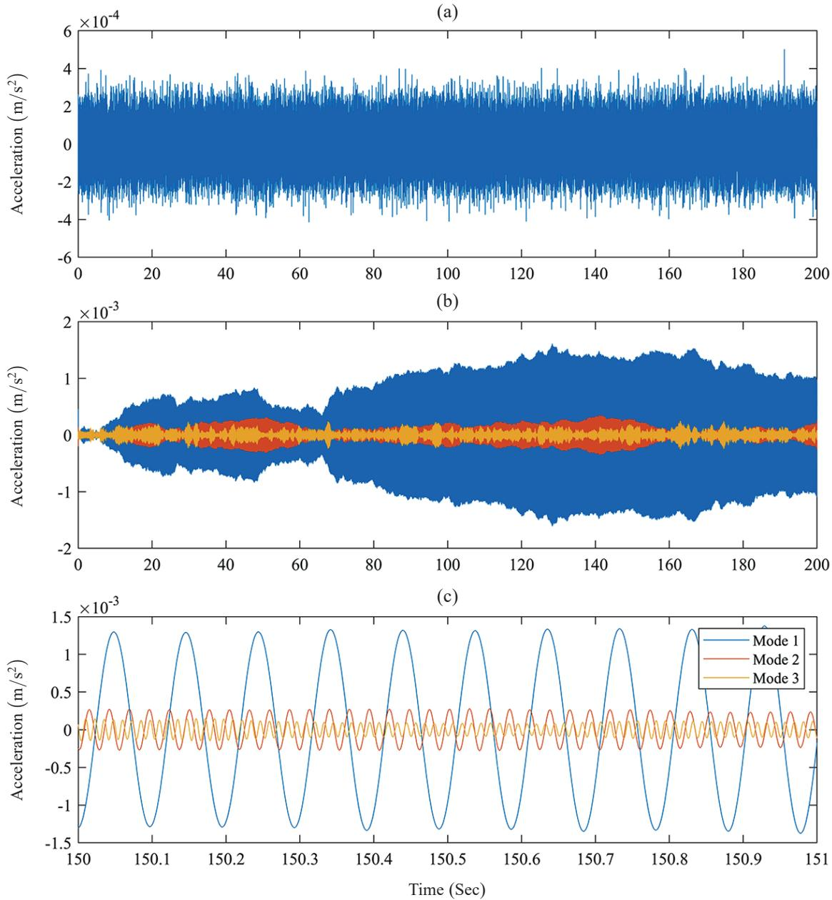
Fig. 2. Dynamic response under ambient base excitation: a) White noise input ambient base excitation, b) Response modal accelerations, c) Enlarged view for modal accelerations for 150 s to 151 s
