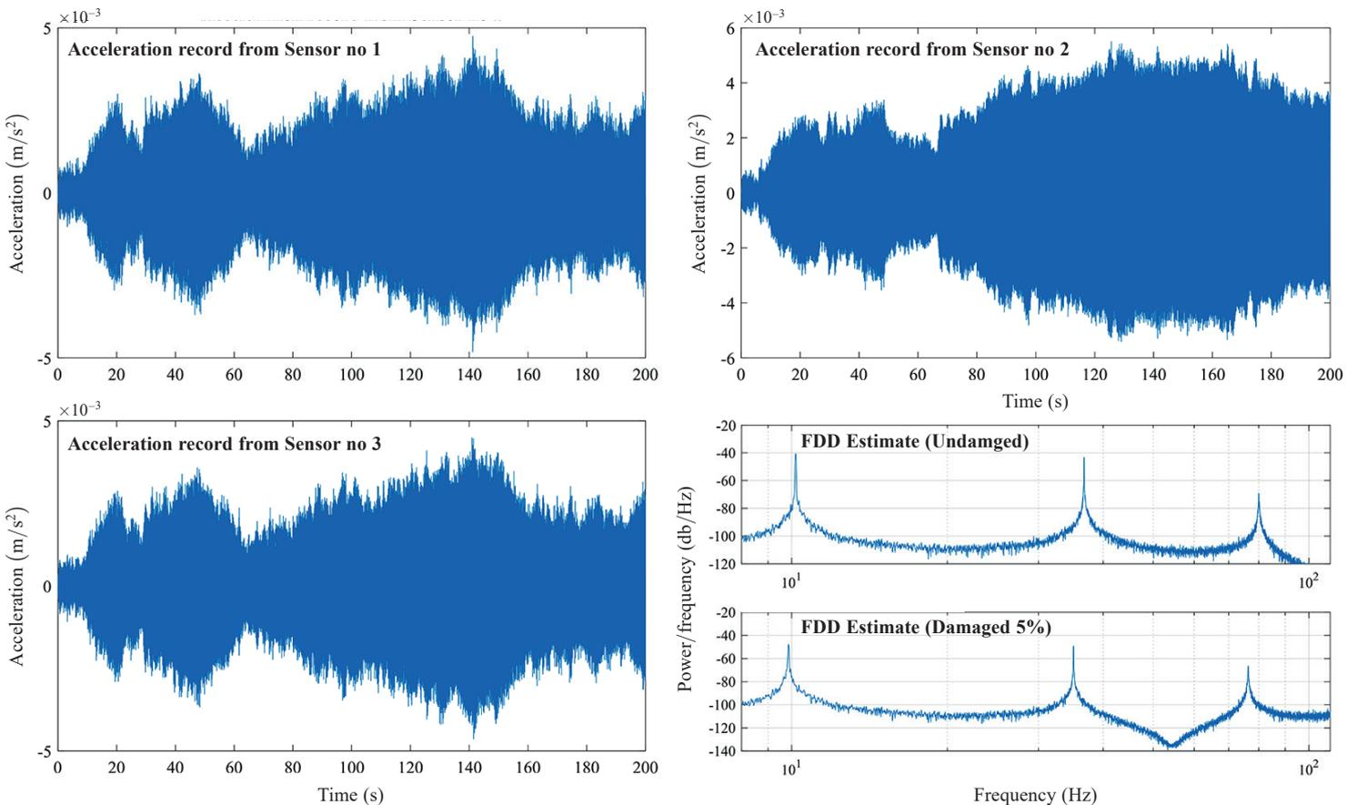
Fig. 5. Acceleration records of undamaged beam and the FDD estimates for undamaged and damaged 5% case of beam
