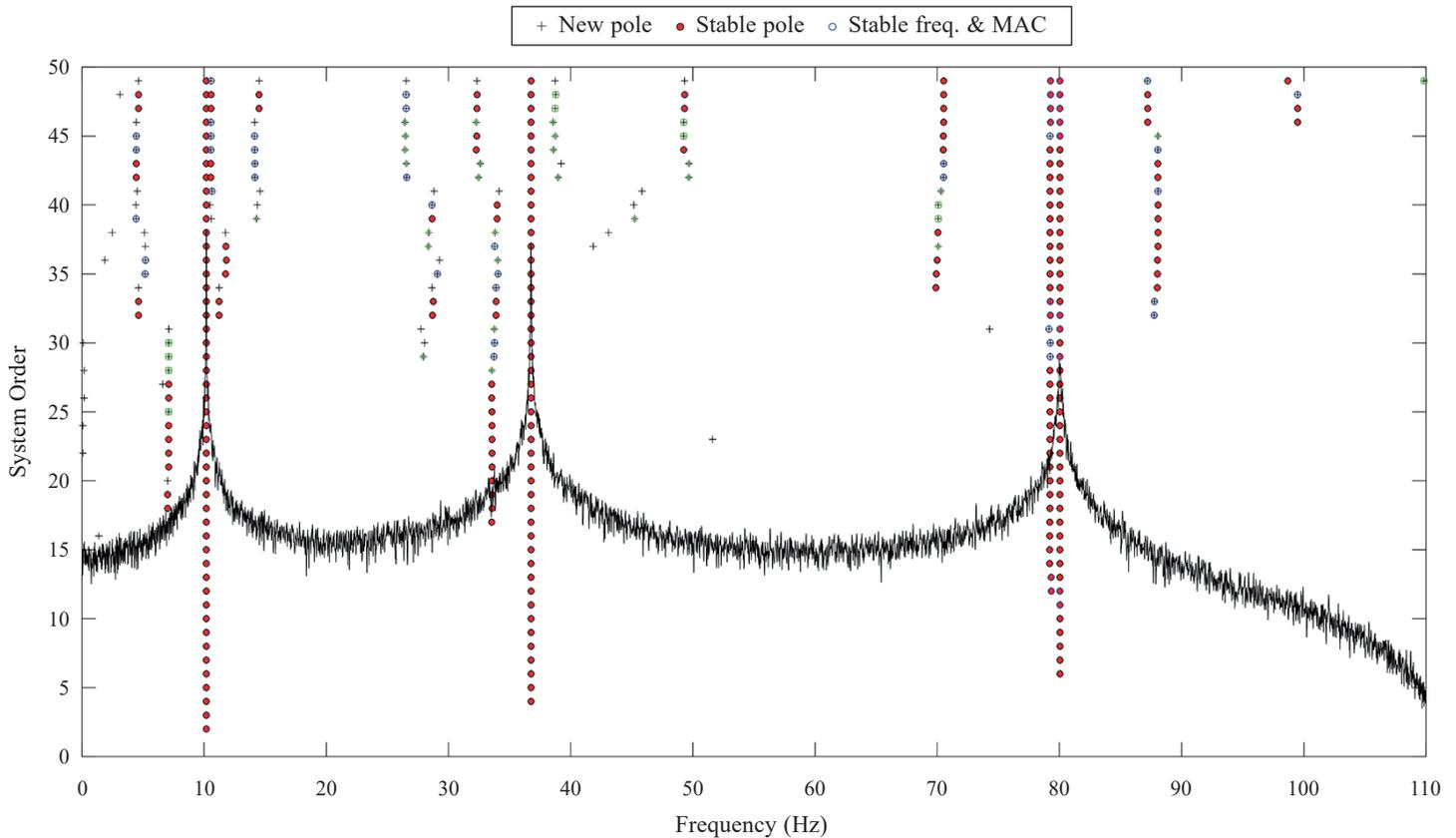
Fig. 6. Stabilization diagram for control beam
