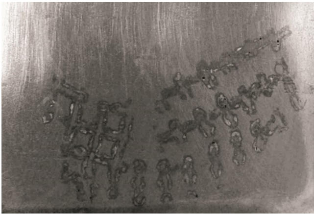
Fig. 3. Casting section with a titanium layer
