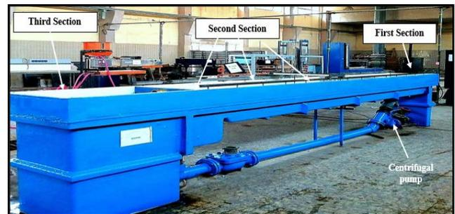
Fig. 2. The laboratory flume; source: own elaboration
