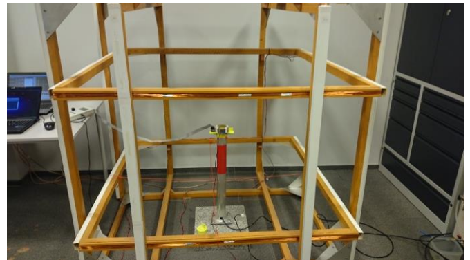
Fig. 6. The three-axial system of the Helmholtz coils eliminating the magnetic field.
