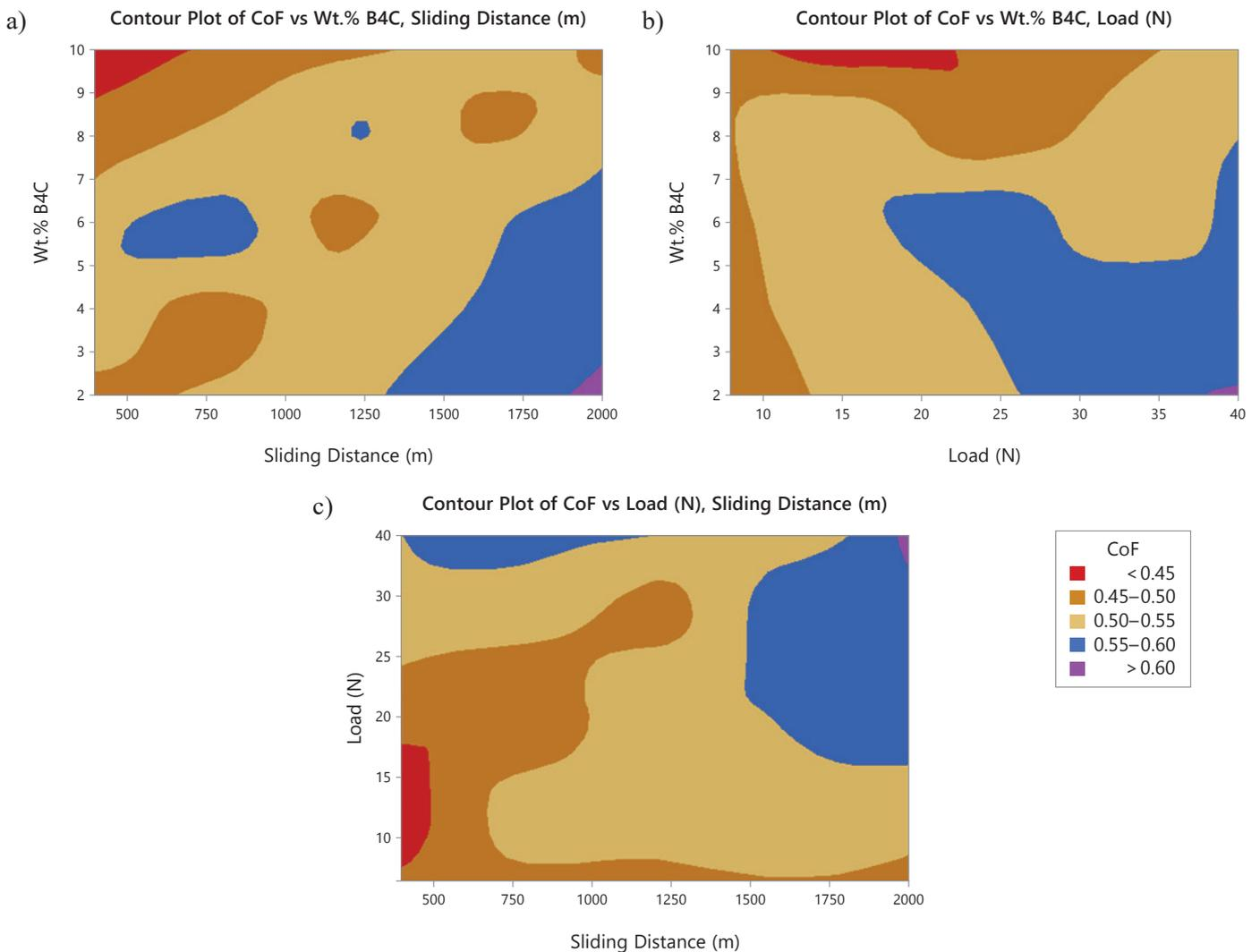
Fig. 5. 2D surface plot of B<sub>4</sub>C wt% and the loads of 8, 16, 24, 32 and 40 N on CoF
