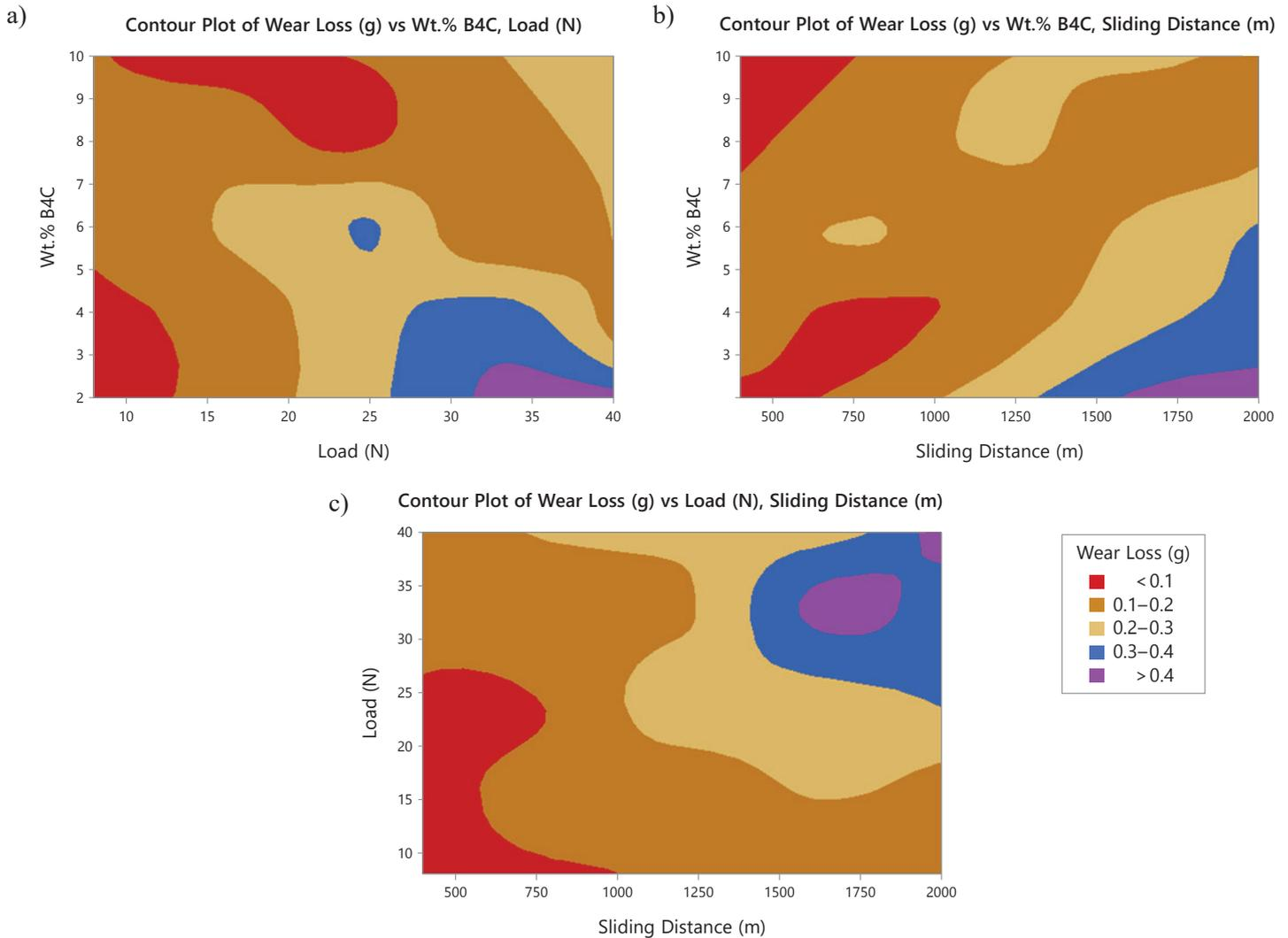
Fig. 6. 2D surface plot of B<sub>4</sub>C wt% and the loads of 8, 16, 24, 32 and 40 N on wear loss
