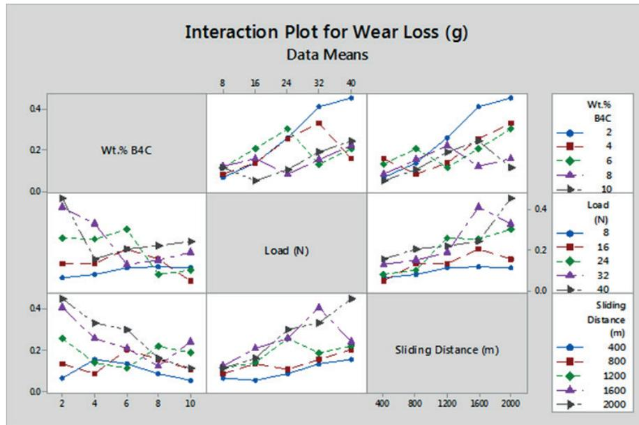
Fig. 3 The interaction plot for wear loss vs wt.%B<sub>4</sub>C, load, sliding distance
