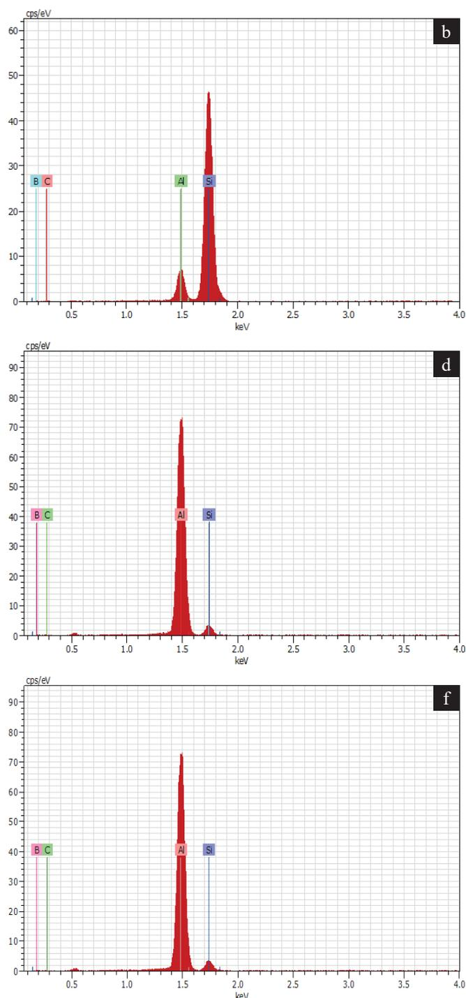
Fig. 2. Mixed powders SEM and EDX analysis of: a-b) Al-Si- $2B_4C$ , c-d) Al-Si- $4B_4C$ , e-f) Al-Si- $6B_4C$  (continued on next page)
