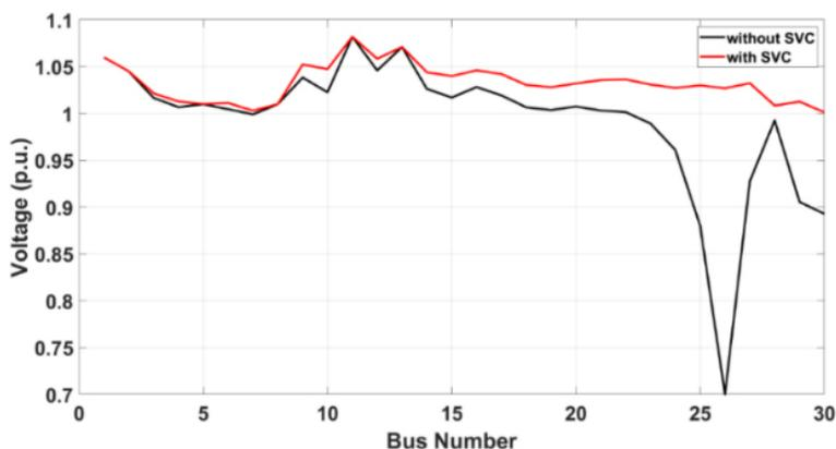
Fig. 7. The voltage profile of the tested IEEE 30 bus system
