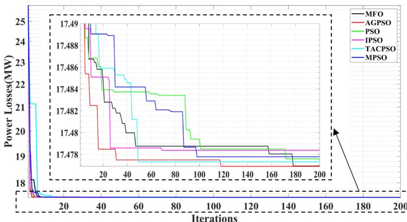
Fig. 6. Convergence curves of all algorithms for the tested IEEE 30 bus system
