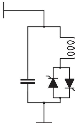
Fig. 1. Schematic diagram of SVC
