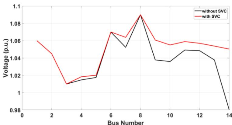
Fig. 5. The voltage profile of the tested IEEE 14 bus system
