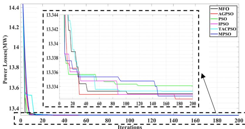
Fig. 4. Convergence curves of all algorithms for the tested IEEE 14 bus system
