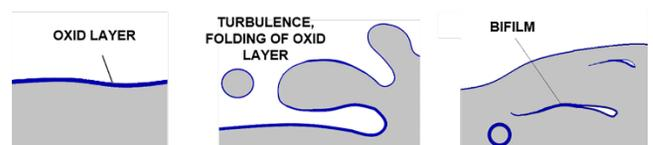
Fig. 1. Scheme of the bifilm creation process
