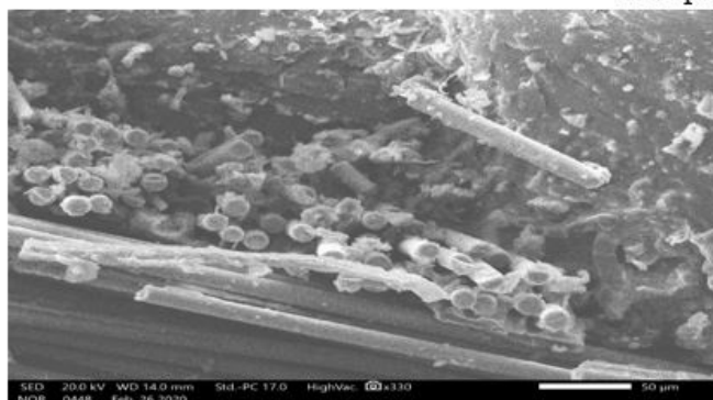
Fig. 6. Fractography analysis on fiber – epoxy with and without carbon particle dispersion in the composite material
