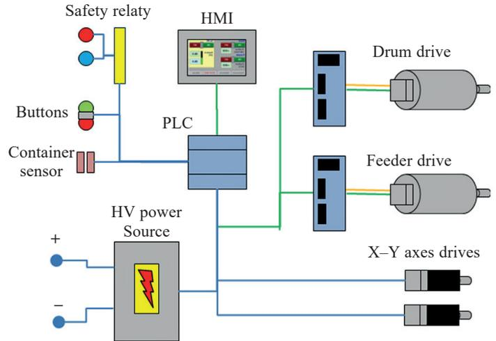
Fig. 6. Schematic view on the control system
