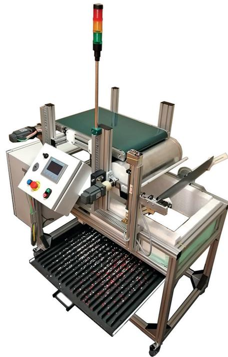
Fig. 5. A prototype of an automated test stand for the electrostatic separation of plastic waste materials
