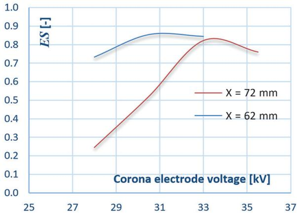
Fig. 7. The influence of the high voltage value on the separation effectiveness coefficient
