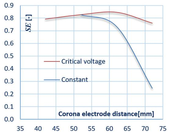
Fig. 8. The influence of the corona electrode position at constant and critical values of the voltage on the separation effectiveness coefficient
