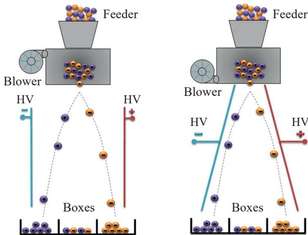
Fig. 1. The typical configuration of free-fall triboelectric separators: a parallel plate (left) and skew plate (right), with an air blower as an example of a tribo-charger
