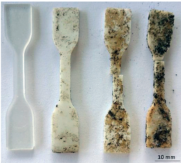
Fig. 4. A macroscopic view of the PLA + 1 wt.% HNT before and after 1, 2 and 3 months of composting
