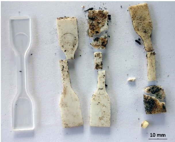
Fig. 3. A macroscopic view of pure PLA: a) before testing, b) after the 1, 2, 3-month composting
