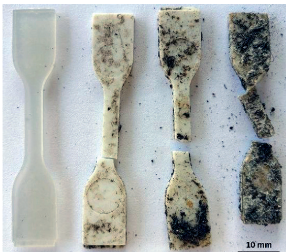
Fig. 5. A macroscopic view of the PLA + 2.5 wt.% HNT before and after 1, 2 and 3 months of composting
