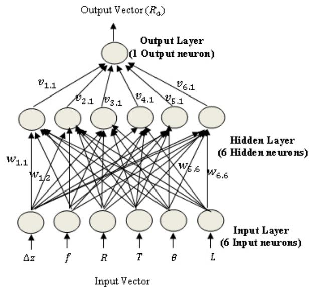
Fig. 1. Structure of three-layer backpropagation neural network
