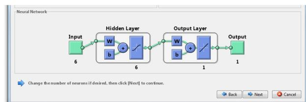
Fig. 2. The network architecture of FFBP
