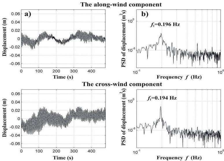
Fig. 18. a) The response of the TV Tower head at the level of  $H = 157$  m (along and cross-wind components) start: 29/04//2011 – 12:02:00, interval 480 s, baseline 501 – 1202, b) Power spectral densities for both components
