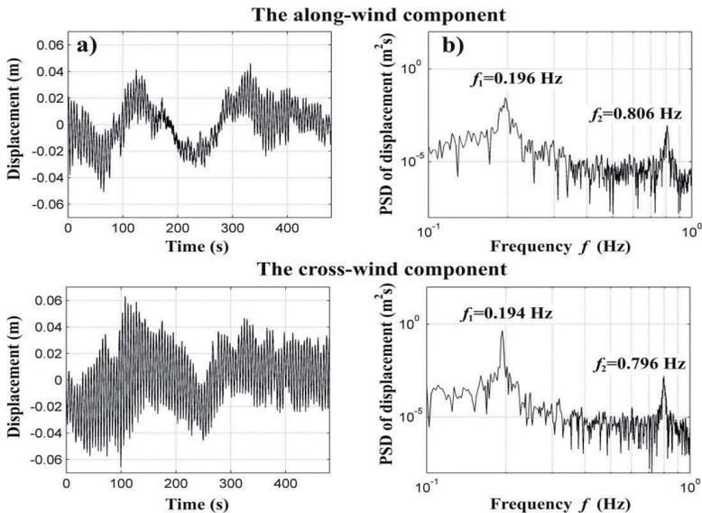
Fig. 16. a) The response of the steel antenna mast tip at the level of  $H = 216$  m (along and cross-wind components), start: 29/04/2011 – 12:02:00, interval 480 s, baseline 501 – 1201, b) Power spectral densities for both components
