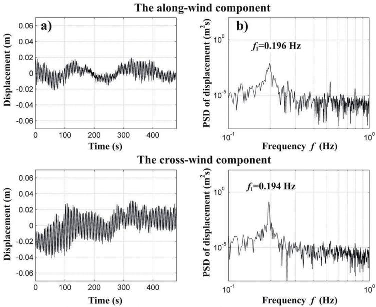
Fig. 19. a) The response of the TV Tower head at the level of  $H = 157$  m (along and cross-wind components) start: 29/04//2011 – 12:02:00, interval 480 s, baseline 502 – 1202, b) Power spectral densities for both components
