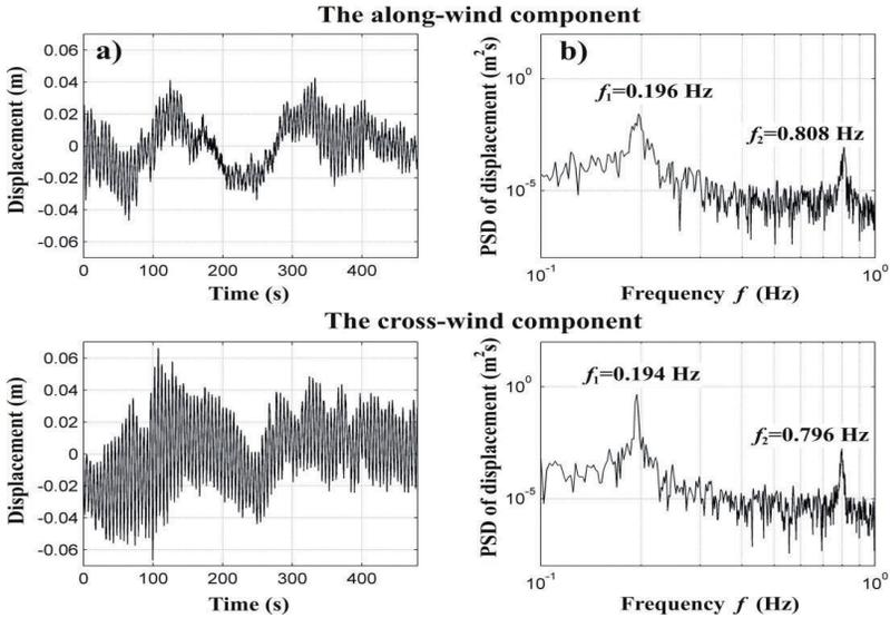
Fig. 17. a) The response of the steel antenna mast tip at the level of  $H = 216$  m (along and cross-wind components), start: 29/04//2011 – 12:02:00, interval 480 s, baseline 502 – 1201, b) Power spectral densities for both components
