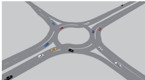
Fig. 8. Simulation scheme of turboroundabout.
