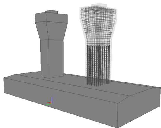
Fig. 7. BIM model of the bridge substructure
