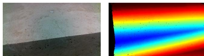
Fig. 1. Data provided by RGB-D camera; RGB image (left) and depth map (right)
