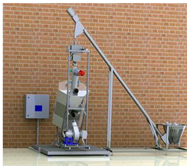
Photo 1. Equipment for frying seeds, nuts, seeds (phot. S. Belozerova)
