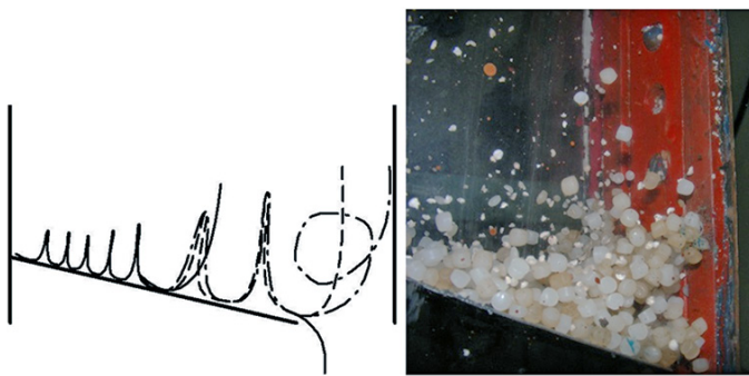
Fig. 7. Second transitional mode of the dryer's operation
