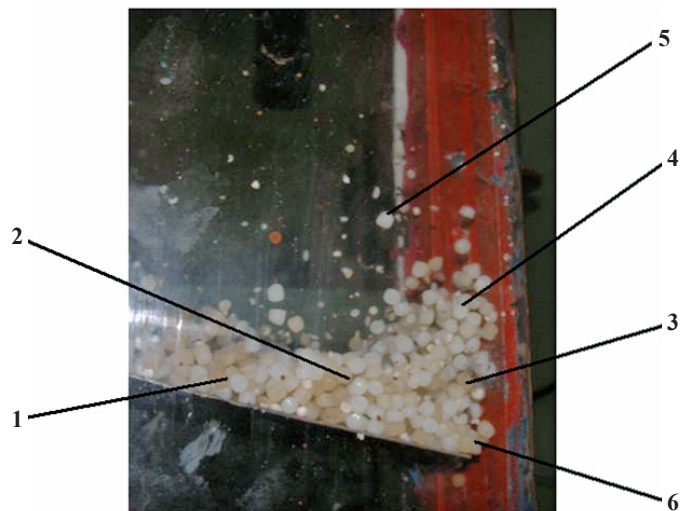
Fig. 6. Distinctive zones of dispersed material motion in the gravitational shelf device: 1 – weighted layer creation zone on the shelf; 2 – zone of lowering the weighted layer intensity; 3 – vortex creation zone; 4 – zone of increased velocity of the dispersed material motion over the outloading gap; 5 – separation zone of finely dispersed material; 6 – outloading zone of the dispersed material from the shelf
