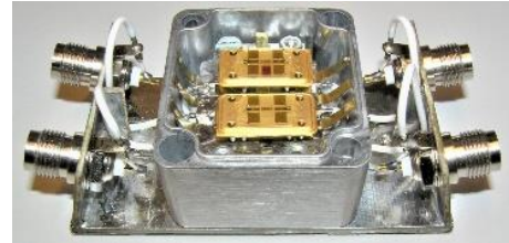
Fig. 7. The practical implementation of the invention of the Patent no. PL 230526 B1 – a measuring chamber for testing using SAW sensors.
