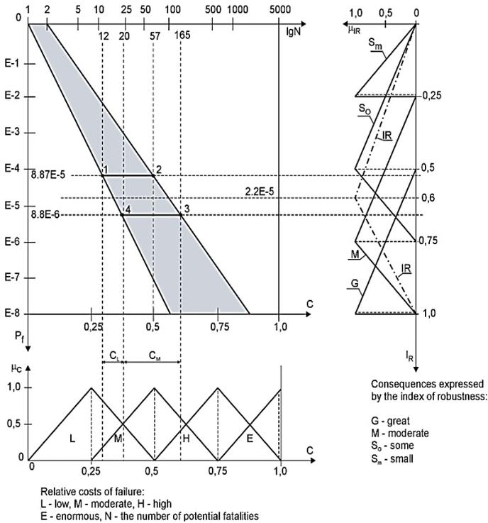
Fig.7. Diagram of frequency-costs-consequences-number of fatalities-robustness (F-C-C-N-IR)
