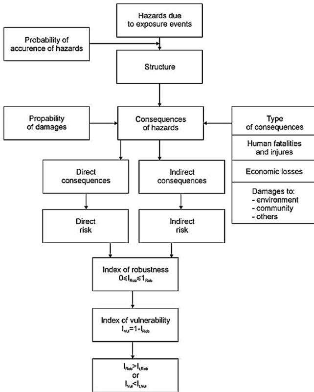
Fig. 1. Overview of risk-based assessment of structural robustness
