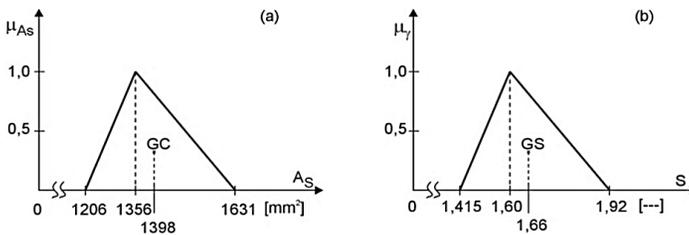
Fig. 5. Membership functions of: (a) required tension steel  $A_s$ , (b) global safety factor  $s$
