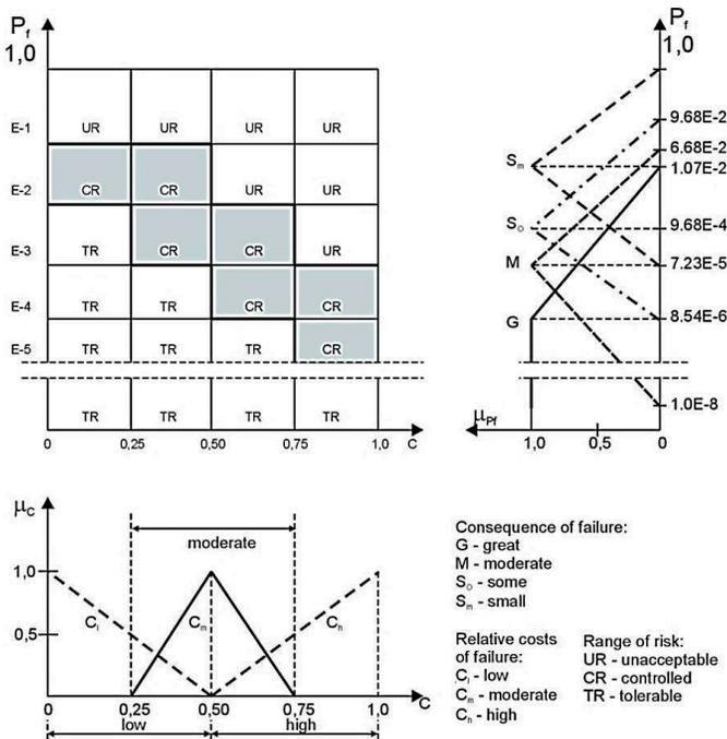
Fig. 3. Frequency-consequence diagram with the fuzzy range limits of structures states. UR-unacceptable risk, TR-controlled risk, NG-negligible risk
