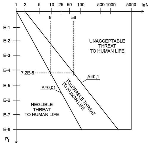
Fig 2.  $F-N$  diagram(on the basis of information contained in [4, 5])
