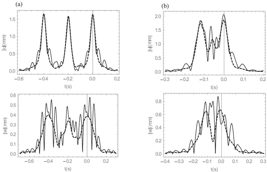
Fig. 7. Double-beam system sensitivity (linear – dashed, nonlinear – solid) in the case of  $V = 50$  m/s,  $k_{Nu} = 10^{15}$  N/m<sup>4</sup>,  $k_{Nw} = 4 \cdot 10^{13}$  N/m<sup>4</sup> and different distances between forces: (a) 10 m; (b) 3 m.
