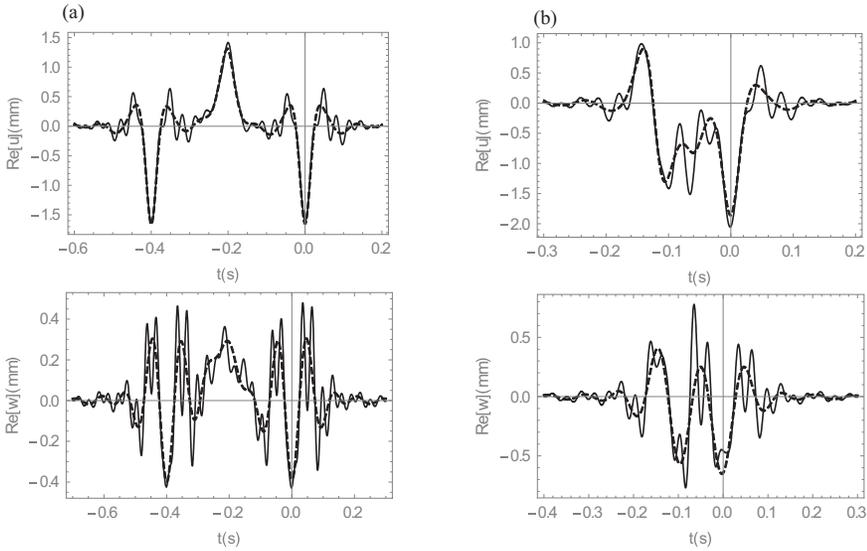
Fig. 6. Vertical vibrations of double-beam system (linear – dashed, nonlinear – solid) in the case of  $V = 50$  m/s,  $k_{Nu} = 10^{15}$  N/m<sup>4</sup>,  $k_{Nw} = 4 \cdot 10^{13}$  N/m<sup>4</sup> and different distances between forces: (a) 10 m; (b) 3 m.
