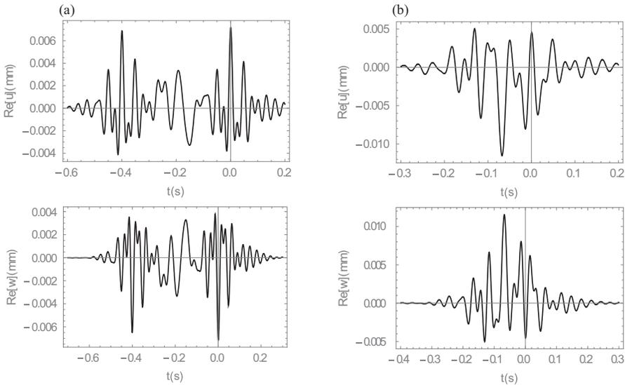
Fig. 8. Second term of Adomian series (Eq. 2.3) ( $V = 50 \text{ m/s}$ ,  $k_{Nu} = 4 \cdot 10^{13} \text{ N/m}^4$ ,  $k_{Nw} = 10^{15} \text{ N/m}^4$ ) for different distances between forces: (a) 10 m; (b) 3 m.
