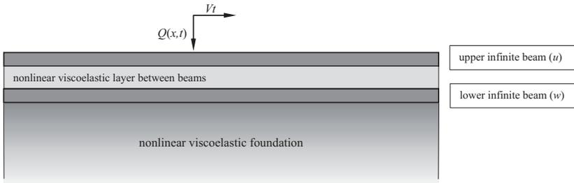
Fig. 1. Nonlinear double-beam model.
