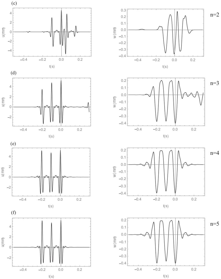
Fig. 2. Successive wavelet approximations (2.1-2.2) of double-beam system vertical vibrations generated by a set of 3 forces acting on upper beam.
