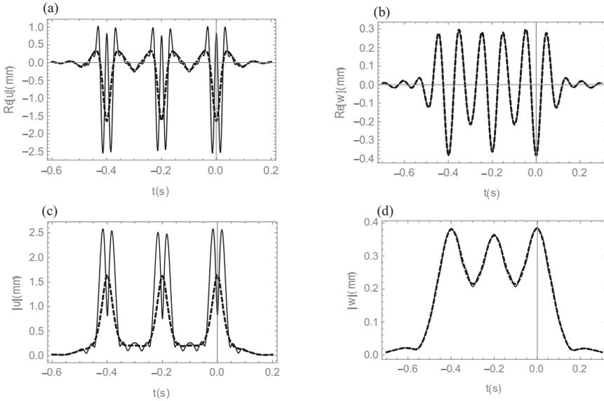
Fig. 4. Vertical vibrations of double-beam system in the case of  $V = 50 \text{ m/s}$ ,  $k_{Nu} = 4 \cdot 10^{13} \text{ N/m}^4$  and  $k_{Nw} = 10^{14} \text{ N/m}^4$ : linear – dashed, nonlinear – solid.
