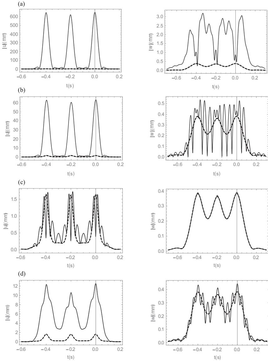
Fig. 5. System sensitivity (linear – dashed, nonlinear – solid): (a)  $k_{Nu} = 10^{16} \text{N/m}^4$ ,  $k_{Nw} = 4 \cdot 10^{13} \text{N/m}^4$ ; (b)  $k_{Nu} = 10^{15} \text{N/m}^4$ ,  $k_{Nw} = 4 \cdot 10^{13} \text{N/m}^4$ ; (c)  $k_{Nu} = 4 \cdot 10^{13} \text{N/m}^4$ ,  $k_{Nw} = 10^{15} \text{N/m}^4$ ; (d)  $k_{Nu} = 4 \cdot 10^{13} \text{N/m}^4$ ,  $k_{Nw} = 10^{16} \text{N/m}^4$ .
