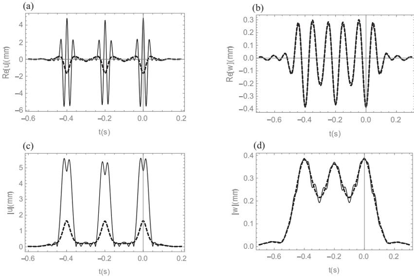
Fig. 3. Vertical vibrations of double-beam system in the case of  $V = 50 \text{ m/s}$ ,  $k_{Nu} = 10^{14} \text{ N/m}^4$  and  $k_{Nw} = 4 \cdot 10^{13} \text{ N/m}^4$ : linear – dashed, nonlinear – solid.
