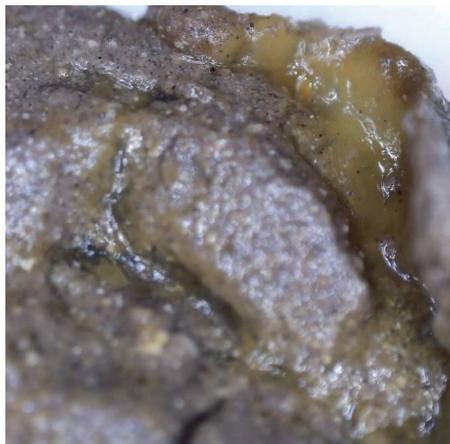
Fig. 4. Hardening slurry surface photographs (magnification of ca. 150x).
