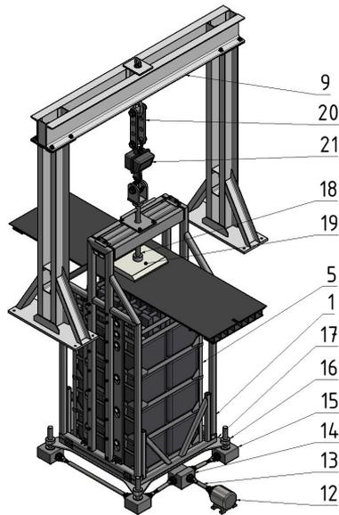
Fig. 3. Equipment with the mechanical lifting of the hanging frame with baskets.
