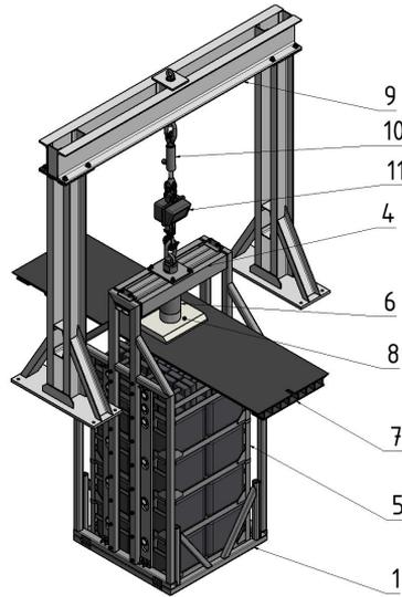
Fig. 2. Equipment with the hydraulic lifting of the hanging frame with baskets.
