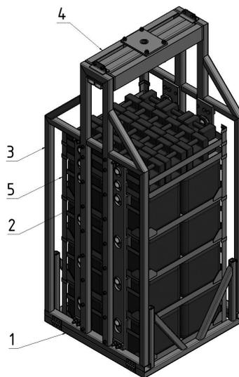
Fig. 1. Hanging frame with baskets with standard weights.
