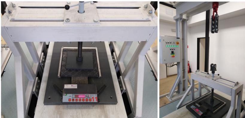
Fig. 4. Test of the axle weighing instrument in the Laboratory for testing of weighing instruments of Slovak Legal Metrology.
