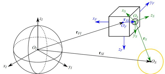
Fig. 2. Sun sensor direction vectors
