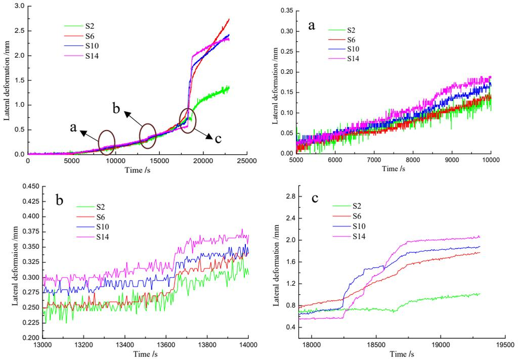
Fig. 10. Lateral displacement time curves of A-D-1 specimen
