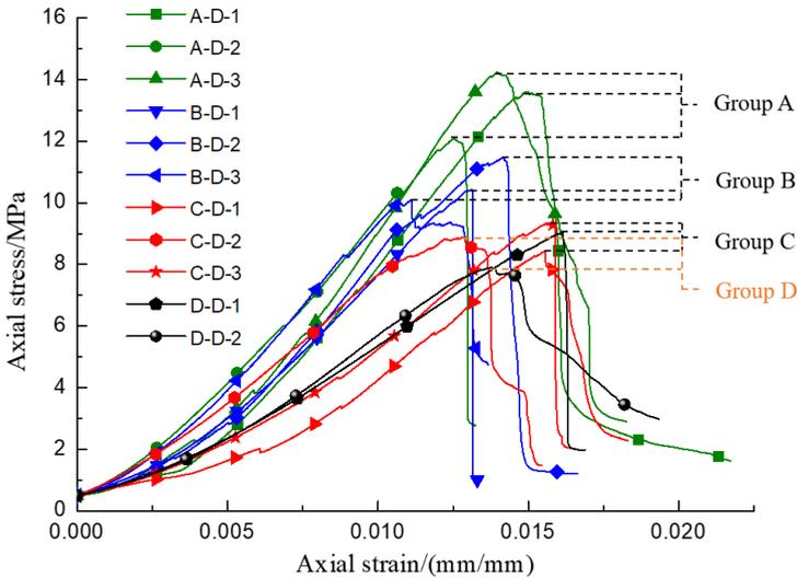
Fig. 7. Stress-strain curves of “roof-strip coal pillar-floor” specimen
