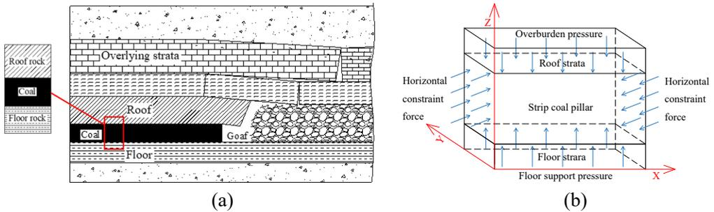
Fig. 2. Schematic diagram of the strip coal pillar mechanical model.
