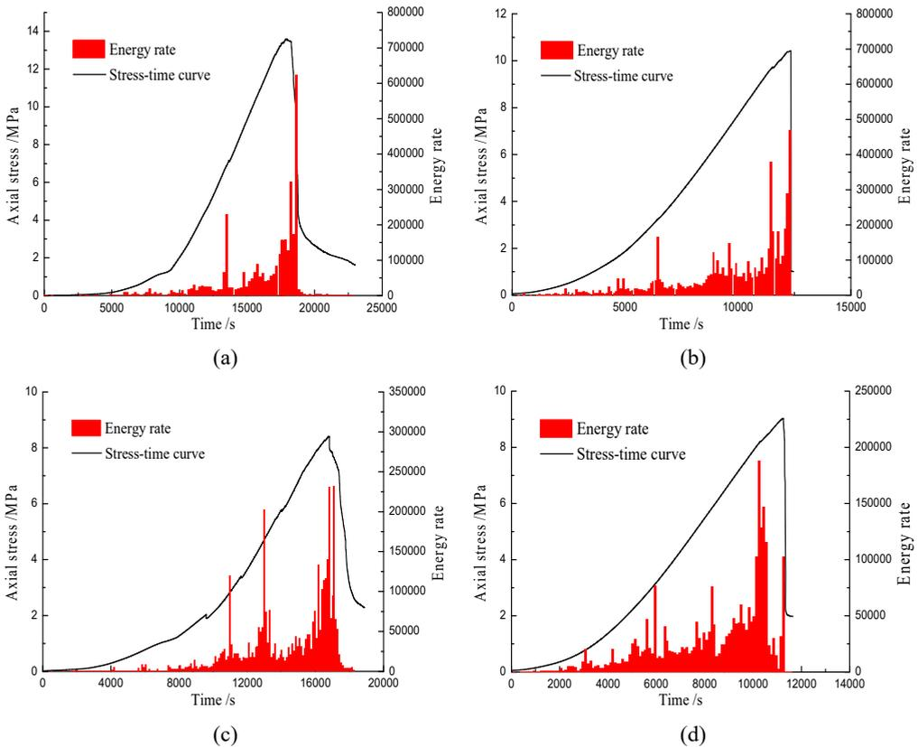
Fig. 12. Stress time and acoustic emission energy rate time curve for strip coal pillar.
