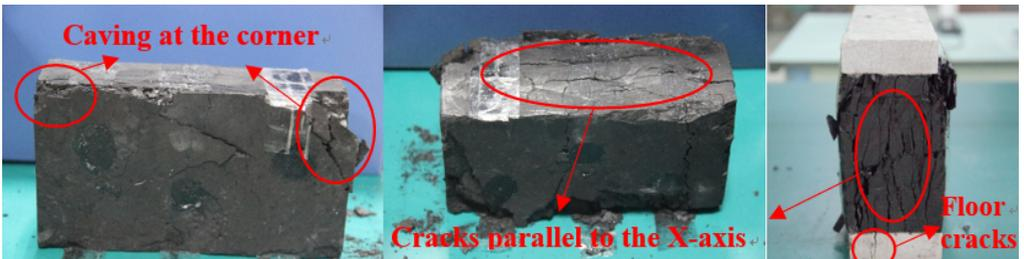
Fig. 11. Failure pictures of test specimens
