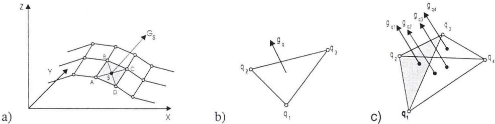
Fig. 3a. a) generated DEM in set S1 with the gradient vector of square; b) the gradient vector of triangle in set S2; c) four normal vectors of triangles built on four chosen points in set S2
