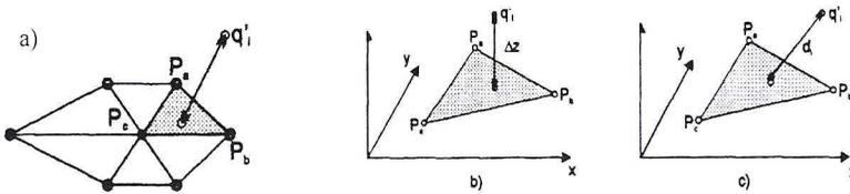
Fig. 1. a) generated surface patches; b) target junction of  $\Delta Z$ -difference; c) target function of distance along surface normal
