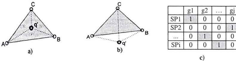
Fig. 2. The point  $q'$  lies on inside (a) and outside (b) of triangle ABC, c) the result of matching process
