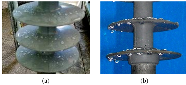
Fig. 2. Drops on the sheds of the silicone insulator after the voltage test (a), drops under the sheds' edges during wetting without the voltage applied (b)
