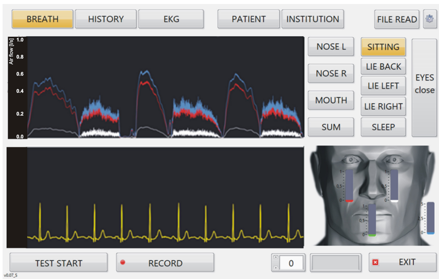
Fig. 8. View of the control panel (virtual control panel of the device generated on the control computer screen) of the NasoOroSpirometer.
