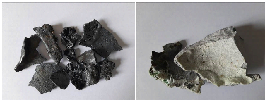
Fig. 3. Steel slag from an EAF (electric arc furnace) on the left, from a LF (ladle furnace) on the right
