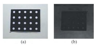
Fig. 9. (a) Chessboard image captured by the RGB camera after calibration.(b) Chessboard intensity image captured by the ToF camera at the same position as (a)
