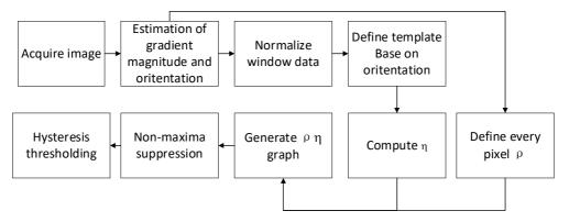
Fig. 3. The flowing chart of embedded edge detection algorithm
