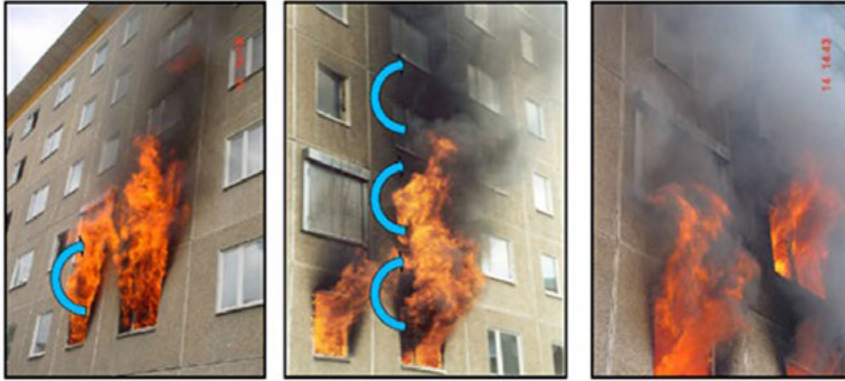
Fig. 4. Development of actual fire acc. to [18]
