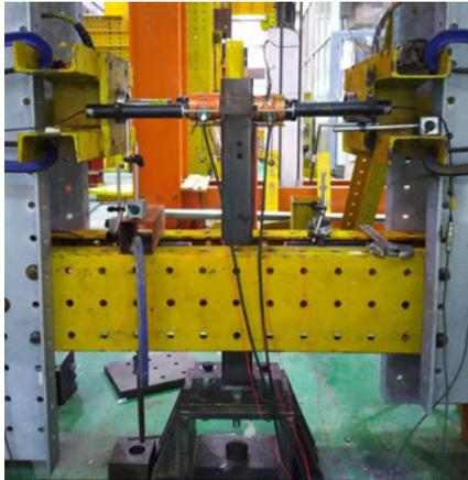
(a) Test setup without axial load
