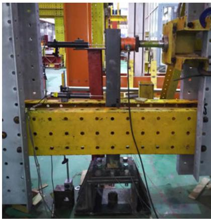
(a) Test setup without axial load
