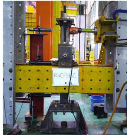
(b) Test setup with axial load
